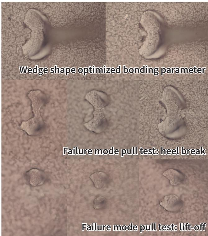
Figure 8: Images of the bonding contacts & failure modes
