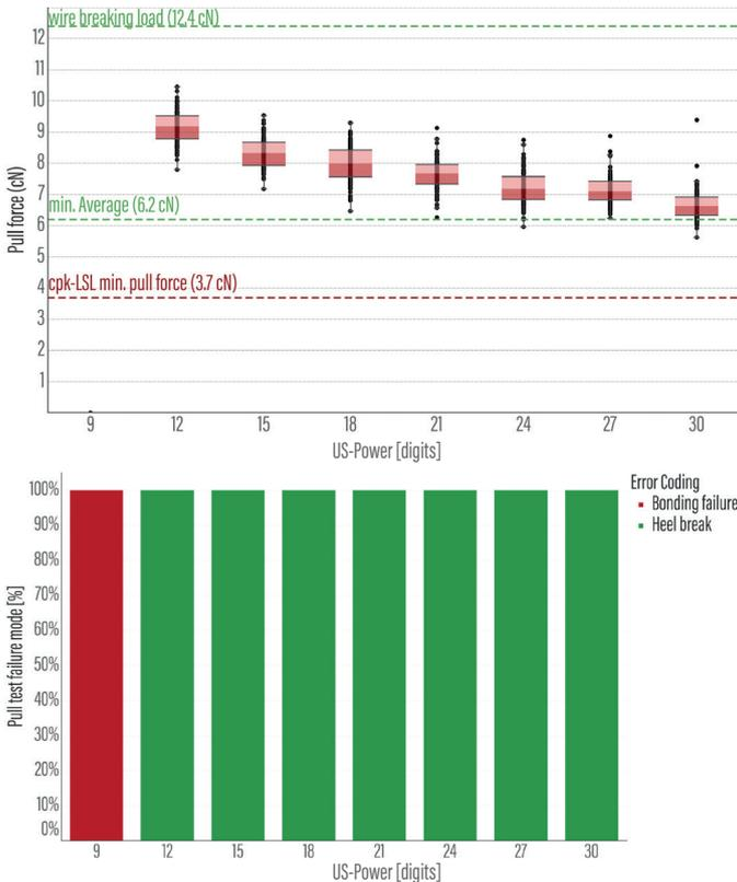
Figure 5: Pull test results  $T_{\text{BOND}} = 130^\circ\text{C}$
