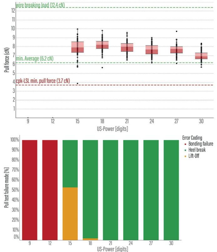
Figure 7: Pull test results  $T_{\text{BOND}} = 90^\circ\text{C}$
