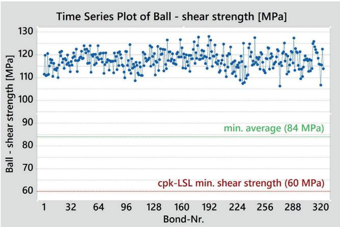
Figure 12: Shear strength analysis  $T_{\text{BOND}} = 150^{\circ}\text{C}$
