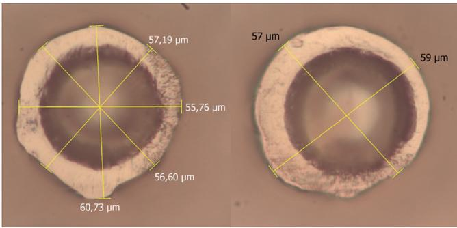
Figure 11: Ball diameter (optimized parameter)
