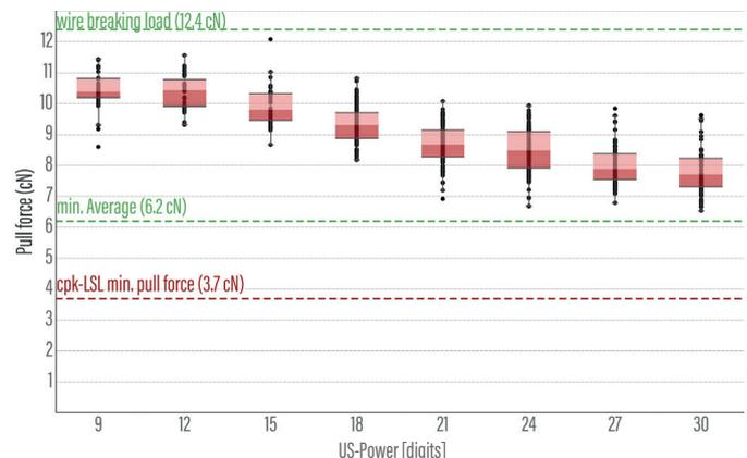
**Figure 3: Pull test results at a bond temperature of 150°C (failure modes: only heel break and lift-off)**
