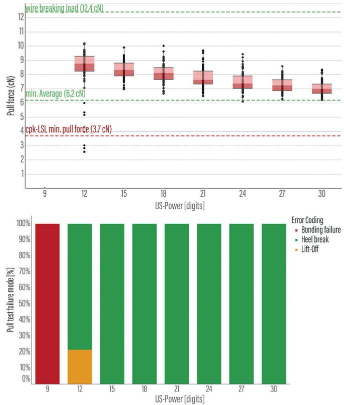
Figure 6: Pull test results  $T_{\text{BOND}} = 110^\circ\text{C}$
