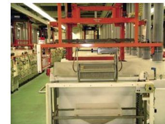
Automatic barrel plating line in the Montblanc plating shop
