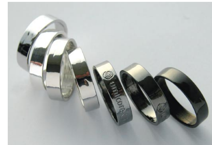
Palladium 457 fits seamlessly into the colour range of white to black sample rings: from left to right RHODUNA® TD, ARGUNA® 621, Palladium 457, Platinum K, Ruthenium 478, Black Ruthenium 477 and RHODUNA® 470 black.
